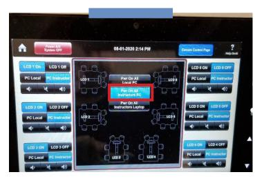
3. Press the **"Pwr On All Instructors PC"** button, and the displays around theroom as well as the podium Wacom monitor should turn on. **Press it oncemore if not all of the displays turn on**.
